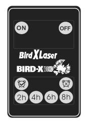
To use the timer, press the remote's TIMER ON button. Unit will flash twice to show it has received the signal. Pressing the TIMER ON button defaults to 2 hours of operation. To select a different duration, press the desired hour button following Timer START. To cancel timer operation, press the TIMER OFF button. Unit will flash twice to show it has accepted the signal.
